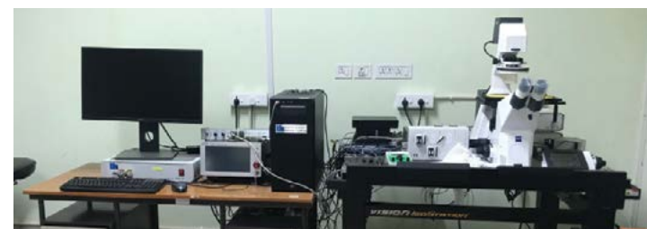
Picosecond Time-Resolved Confocal Microscope with Single Molecule Sensitivity
