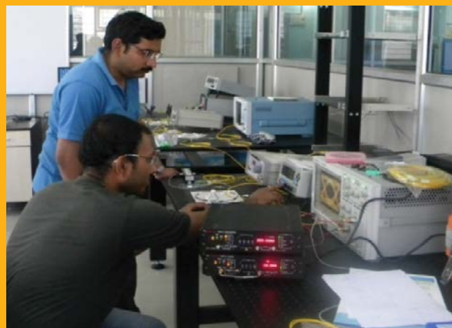
Optical Communication Lab:- WDM DFB laser sources, Optical spectrum analyzer, Digital Sampling Scope with Precision Time Base Module for signals up to 12.5Gbps, 0.5Gbps-12.5Gbps PRBS generator and Bit Error Detector, Optical Network Simulator: OPNET, Device
