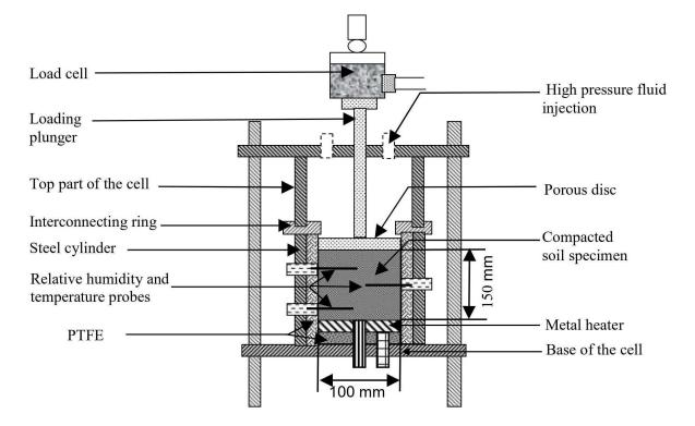
Fig.1. Schematic diagram of the proposed thermos-hydraulic cell
