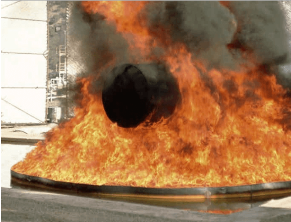
Fig. 1.3 Large circular cylinder engulfed in a pool fire (Kramer et al. , 2003)
