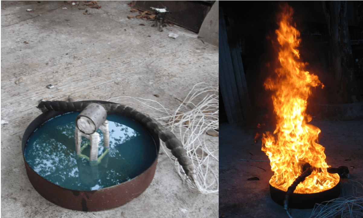
Fig. 6.2 Horizontal cask engulfed in 0.7 m diesel pool fire
