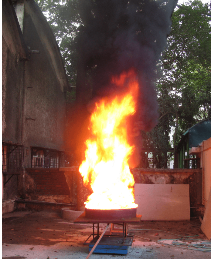
Fig. 3.1 Experimental setup of 0.3 m pool fire with weighing machine
