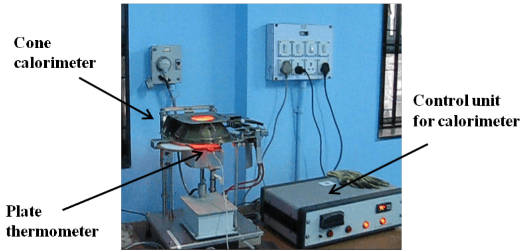
Fig. 6.6 Curing of plate thermometer under cone calorimeter (heater is ON)
